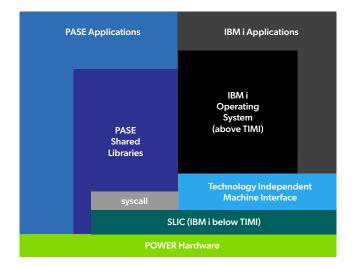
As one can see from the diagram, PASE runs on top of the same hardware as IBM i and programs running within PASE have access to IBM i items such as Db2 resident data, programs (RPG, Cobol, CL), commands, data areas, and data queues (to name a few) via the syscall interface between PASE and the TIMI layer of IBM i.
